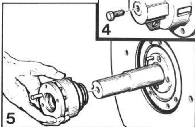
Note that seal drive pin is located over the shaft keyway. If the seal is to be replaced, push new seal on to shaft and reverse the preceding steps. Be sure that the seal drive pin extends into the hole above the keyway in the drive yoke.
