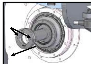
**NOTE: Use caution to avoid damage of Lip Seal when removing MECHANICAL SEAL.**
