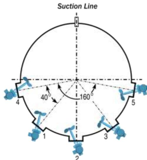
Locating the mixer(s) at the opposite side of the Suction Line the allows the user to take advantage of the natural cleaning that will occur due to product being drawn from the tank.
