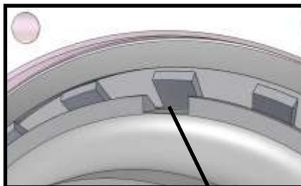
NOTE: TAB may not be in locked the 0° position and may be reinstalled in any of the 8 locking positions.
