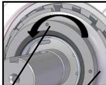
9. Partially thread in 1/4-20 bolts (shown with arrows) to aid in turning RETAINING RING with screwdriver.
