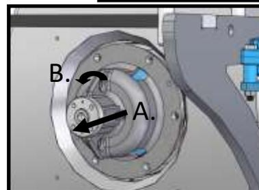
4. Drain RESERVOIR by removing the plug and open the release VALVE HANDLE. A
